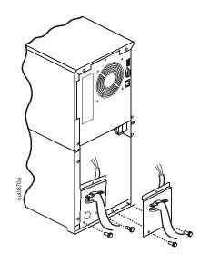
Secure the terminal block and label to the UPS with two screws (supplied), as shown in the diagram.
