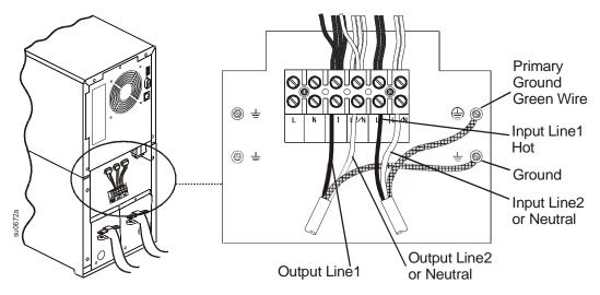
Connect the terminal block and UPS connectors as shown in the diagram.
