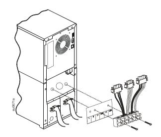
Refer to the diagram below. Use the screws supplied. Connect the ground wires with the grounding screws. Connect the input and output cables.
