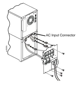
Secure the replacement input and output panels (supplied), to the UPS. Secure the panels with four of the screws removed from the factory installed PDU panel.
