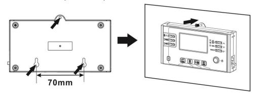
**Note:** Installation to the wall should be implemented with the proper screws. Refer chart for recommended spec of screws.
